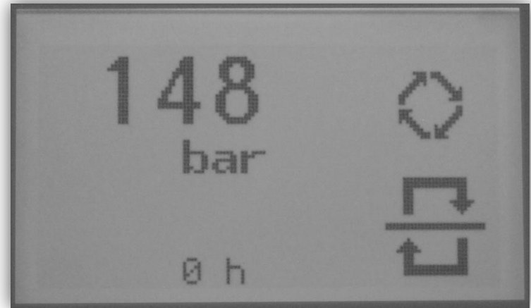
Main Display (compressor running, fully automatic)
